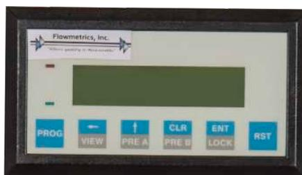
Rate/Totalizers are available to work with most flowmeter types and most common electrical signals produced by flowmeters. In some cases an amplifier or signal conditioner may be necessary. Non-linearity corrections are available in some units. Separate K-factors (calibration points) can be programmed to compensate for changes in K-factor with flow rates. Linearization is useful in improving the accuracy of the flowmeter.
