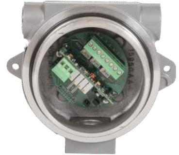
Signal conditioners are secondary devices intended to amplify, filter, condition, scale, and convert low level "raw" signals produced by many transducers and convert it into the desired industry standard high level signal prior to transmitting it across potentially noisy environments. In some cases, a secondary function is providing signal isolation.
